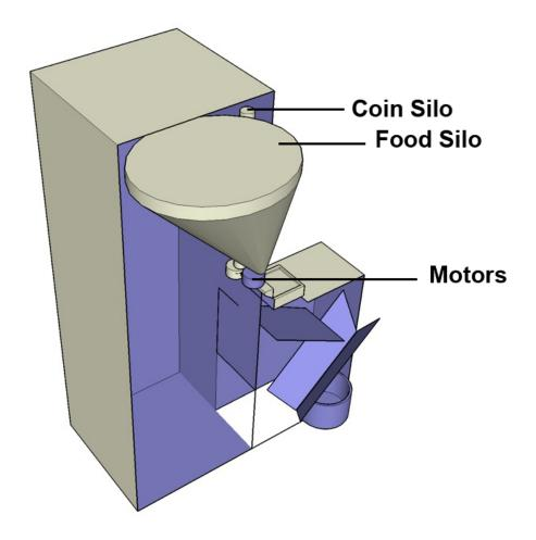
Here the gross inner components are described; the tube containing coins, the food hopper (designed for easy removal and replacement to speed the stocking process), and the motors which drive the dispersal of both onto the food tray. Note that this uses the standard "gravity feeder" methodology common to most commercial feeding mechanisms. This is to prevent clogging and jamming of the device and also to keep the overall design as simple as possible for maintenance and production purposes.
